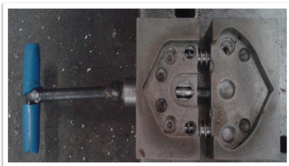
Figure no.1 Fixture of component for milling operation
